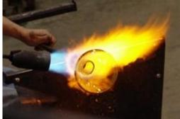
First, glass can be improved by a factor of up to 10 by treating the glass with heat or chemicals so that the outer surfaces are compressively stressed at relatively high levels. This causes the cracks to be "held closed" by the continuous residual stress. This is called tempering or tempered glass. Second, the glass can be kept away from anything that could scratch the surface.
